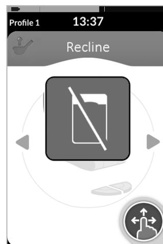
The user must finish the current action to change the function. Otherwise, a function change blocked overlay displays.
