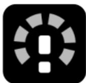
Speed reduction is shown in the display. If the elevating seat is raised above a certain point, an icon with an exclamation point displays in the status bar. This indicator remains active until speed reduction is deactivated by lowering the elevating seat.
