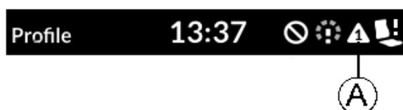
Additionally, the status LED inside the ON/OFF button flashes red. The number of flashes matches the number in the fault icon in the status bar.
