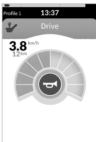
As soon as you start driving, the speed slider and Navigation button disappear from the display. The current speed on the speedometer, if it is enabled.
