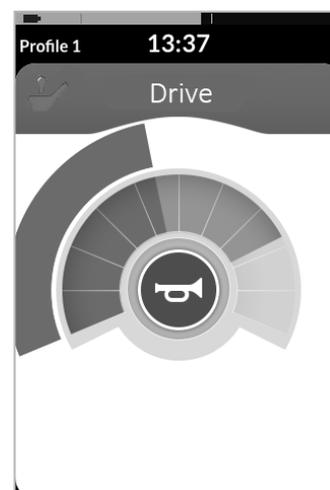
The speedometer/odometer display is a new feature introduced for LiNX MR6.0. It replaces the sweeping speed gauge that wrapped around the speed dial.
