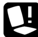
An icon with a seat and an exclamation point displays in the status bar. This icon remains active until the elevating seat lockout is deactivated by moving the seat tilt or recline up.
