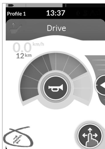
In this mode, you can step up or down through one of five fixed speeds. The speeds available are 20%, 40%, 60%, 80% and 100% of the maximum preset reverse or forward speed <sup>Ⓐ</sup> of the selected drive screen. The speed is maintained for the programmed Latch Drive Timeout period as long as no further command is given.
