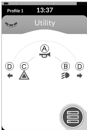
2. Give input to the front **A** to turn on the horn.
