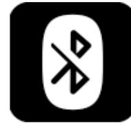
The disabled Bluetooth functionality is indicated by an icon in the status bar and the status LED inside the ON/OFF button pulsing for a duration of six seconds.
