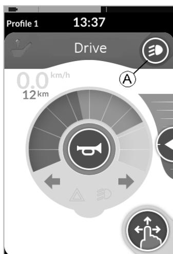
2. Tap the left turn signal symbol **B** or the right turn signal symbol **C** to turn off the turn signal.
