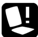
An icon with a seat and an exclamation point displays in the status bar. The icon remains active until the tilt limit is deactivated by lowering the elevating seat.
