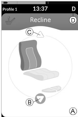
When a motion becomes active, the Navigation button disappears (A), the active direction of the motion (B) displays, the other direction becomes inactive (C) and the Drive Lockout icon (D) displays in the status bar.
