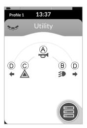
2. Give an input to the front (A) to turn on the horn.
