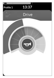
The speedometer/odometer display is a new feature introduced for LiNX MR6.0. It replaces the sweeping speed gauge that wrapped around the speed dial.
