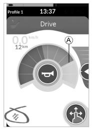
In this mode, you can step up or down through one of three fixed speeds. The speeds available are 33%, 67% and 100% of the maximum preset reverse or forward speed (A) of the selected drive screen. The speed is maintained for the programmed Latch Drive Timeout period as long as no further command is given.
