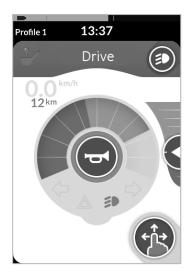
If you start driving, the Lighting button panel overlay closes, and the position lights remain turned on.
