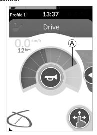
In this mode, you do not have fixed steps and can choose the latched speed yourself. The speed is maintained for the programmed Latch Drive Timeout period as long as no further command is given.
