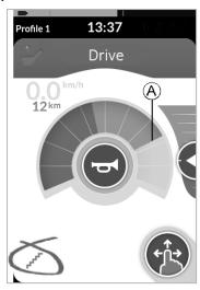
In this mode, you can step through one of five fixed speeds. The speeds available are 20%, 40%, 60%, 80% and 100% of the maximum preset reverse or forward speed A of the selected drive screen. The speed is maintained for the programmed Latch Drive Timeout period as long as no further command is given.
