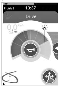
In this mode, a single drive command (forward or reverse) causes the wheelchair to accelerate to the maximum drive speed (a) of the selected drive screen and remain at that speed for the programmed Latch Drive Timeout period as long as no further command is given.
