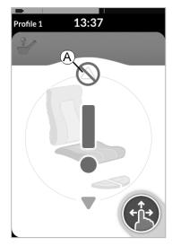
The seating electronics are equipped with an elevating seat lockout switch to prevent the elevating seat from rising above a certain point when the seat tilt or recline is adjusted above a certain point. The seating electronics stop automatically, a grey exclamation point displays on the seating screen and extend is inhibited **(A)**.
