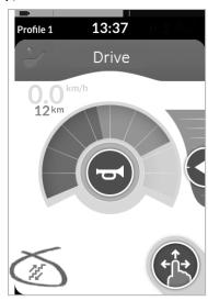
In this mode, you can step up or down through one of five fixed speeds. The speeds available are 20%, 40%, 60%, 80% and 100% of the maximum preset reverse or forward speed (A) of the selected drive screen. The speed is maintained for the programmed Latch Drive Timeout period as long as no further command is given.
