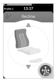
Seating screens are used to operate the seating functions. Refer to 6.16.1 Through Seating Screens, page 54.
