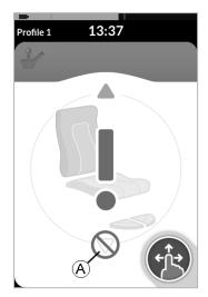
The maximum tilt limit switch functions to prevent the seat tilt or recline from extending beyond a maximum preset angle when the elevating seat is raised above a certain point. The seating electronics stop automatically, a grey exclamation point displays on the seating screen and tilting or reclining backward is inhibited **(A)**.
