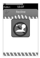
When a system is powering up or after a function change, no direct access switches can be active; otherwise, a seating OON warning displays.
