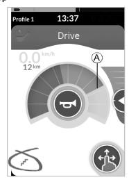
In this mode, you can step through one of three fixed speeds. The speeds available are 33%, 67% and 100% of the maximum preset reverse or forward speed (a) of the selected drive screen. The speed is maintained for the programmed Latch Drive Timeout period as long as no further command is given.
