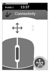
Connectivity screens allow you to communicate with external devices. The connectivity function included on your remote is a mouse mover. The mouse mover allows you to control the cursor on a PC or laptop screen with a user input on the wheelchair, such as the joystick on the remote module or buttons connected via control inputs. For more information about Connectivity screens and how to use them, refer to 6.17 Using Connectivity Screens, page 59.
