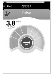
As soon as you start driving, the speed slider and Navigation button disappear from the display. The current speed on the speedometer, if it is enabled.
