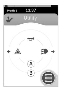
By default, this function is enabled only for chair configurations with an external control input that will not allow the control of the horn or lights. Contact your provider to change the configuration and to set your desired operations.
