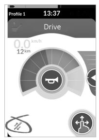
Each drive function can be assigned with a latched driving mode by your provider. The six latched driving modes, which are indicated on the lower left of the drive screen, and their corresponding symbols are listed in the following table.
