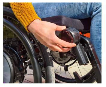
One click on the control unit is all it takes to switch to Cruise Mode while driving.
